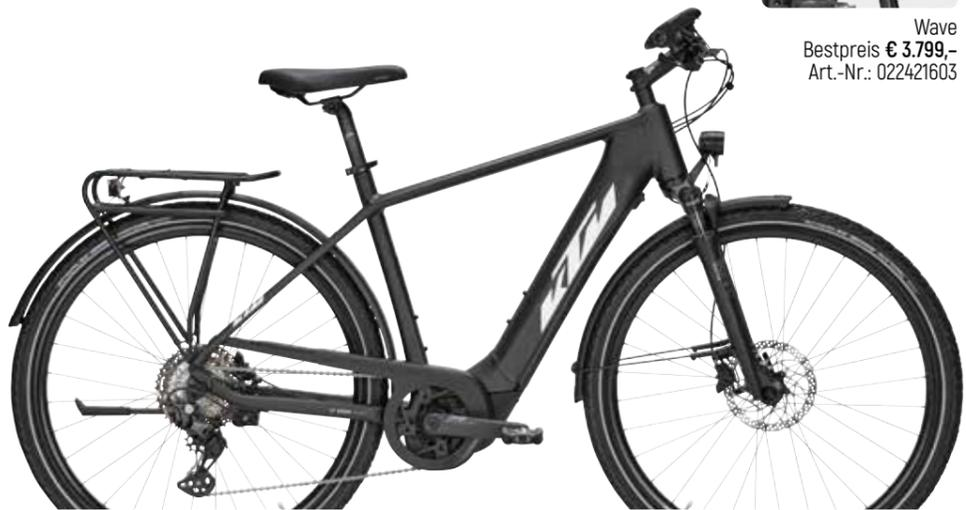
SHIMANO Deore 10-Gang Schaltwerk | Performance Line CX GEN4 Mittelmotor, Akku: 625 Wh | blockierbare SR SUNTOUR NCX-D Federgabel
